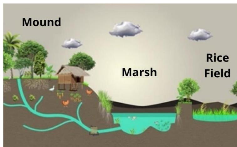
*The key principle of the Khok Nong Na Model is to store sufficient water by focusing on storage of water in three main areas: mound, marsh, and rice field.*
